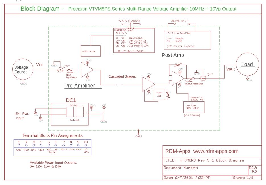
**Insufficient input shielding applied to the VTVM module could increase the noise-signal ratio which could result in VTVM input or output inaccuracy.** Default VTVM power input(s): +4.9VDC to +9VDC
