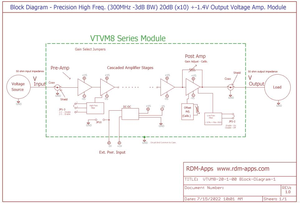
**Insufficient input shielding applied to the VTVM module could increase the noise-signal ratio which could result in VTVM input or output inaccuracy.** Default VTVM power input(s): +4.9VDC to +9VDC
