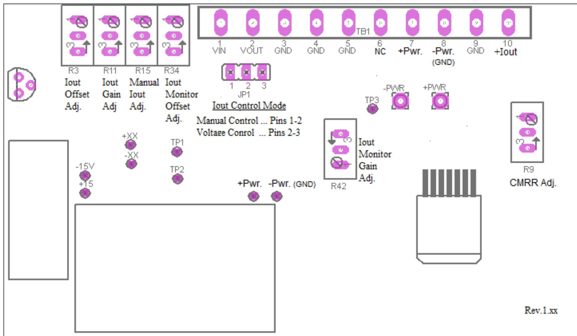
**RDM-Apps** Setup – PCB Revs.1.xx - CSE CSE00GL-100-xx-20V-BFL Constant Current Source / Sink Module.
