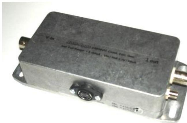
**RDM-Apps Setup – PCB Revs.1.xx - CSE CSE00GL-100-xx-20V-BFL Constant Current Source / Sink Module.**
